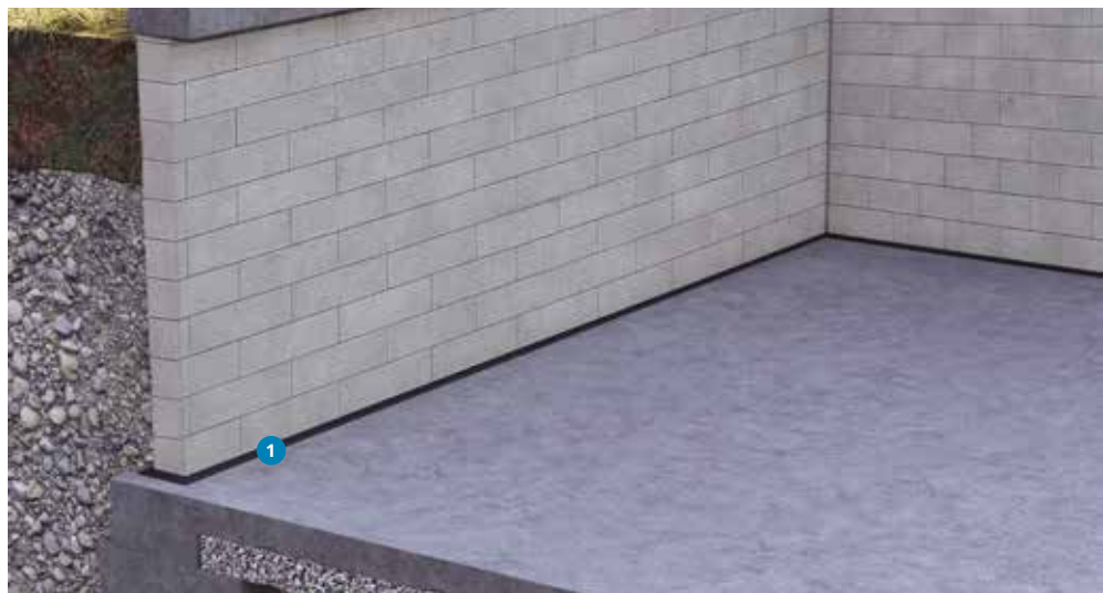
1 Horizontal barriers for walls KÖSTER Fix-Tape 15 SY
