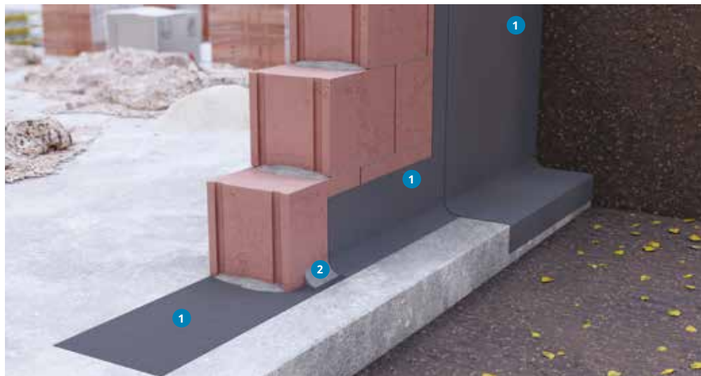
1 Horizontal barriers for Waterproofing Layer (different options) KÖSTER NB 1 Grey KÖSTER NB 4000 KÖSTER NB Elastic Grey
