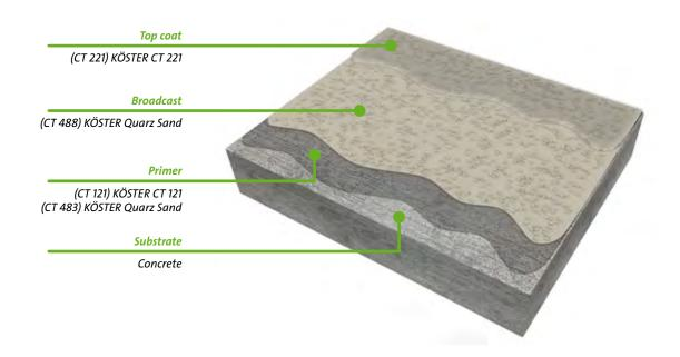
Parking garages and trafficked areas have especially high requirements on coatings. The KÖSTER OS 8 System is a highly resistant, easy to apply solution.
