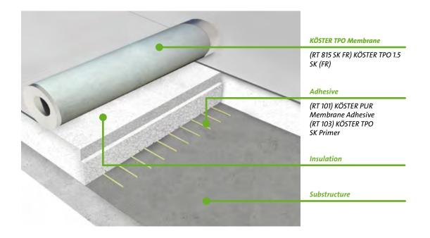
The self-adhering layer guarantees immediate, long-term adhesion and provides maximum protection against wind suction forces. The safe and easy welding of the overlaps with a hot air gun complete the installation advantages of the KÖSTER TPO SK (FR) single layer roofing system. Hardly any other material is as well suited for the waterproofing of roofs as thermoplastic polyolefin (TPO).
