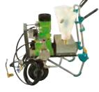
*Electrical 2C injection pump with stageless adjustable* mixing ratio (gel : water). Operating pressure is approx. 30 bar. The maximum delivery rate is approx. 2.51/min.
