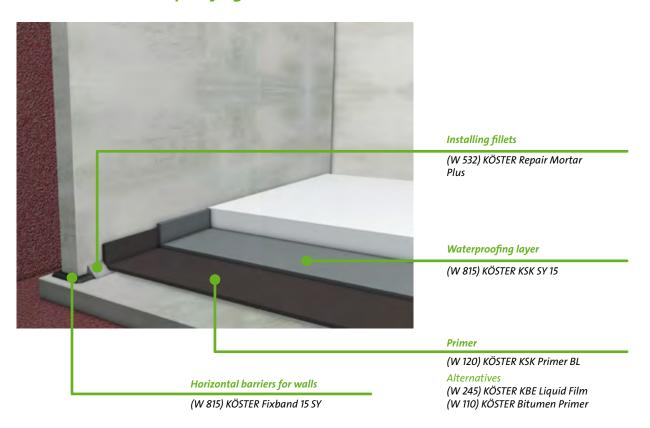
Fast, easy application without long waiting times: Waterproofing of the floor slab with KÖSTER KSK cold applied, self adhesive waterproofing membranes.
