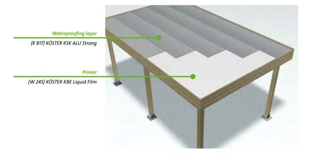
Smaller roofs on non residential buildings can quickly and easily be waterproofed with the cold self-adhesive sealing membrane KÖSTER KSK ALU Strong. The clean and dry substrate is primed with KÖSTER KBE Liquid Film. KÖSTER KSK ALU Strong is applied onto the dry and primed roof area. Membranes have to overlap a min. of 10 cm on each side. Connections, penetrations and overlaps are sealed with KÖSTER KBE Liquid Film.
