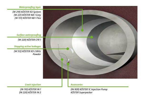
The method for waterproofing tunnels with KÖSTER products is based on a combination of negative side waterproofing and a liquid applied crack bridging waterproofing compound. The waterproofing layers cannot be infiltrated and the water will not move laterally between the layers as with membranes. The system does not need drainage. No water is being drained off the surrounding soil so the water table is not affected.
