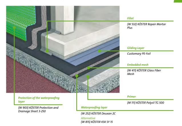
A complete waterproofing system in new construction includes waterproofing the floor slab. Compared to the application on top of the concrete slab the installation of the waterproofing layer underneath the foundation plate keeps the foundation dry and the concrete provides a better thermal insulation.
