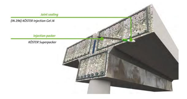
For the injection of expansion joints (pictured here in an underground parking garage ceiling above a support beam) usually a small number of injection packers are sufficient. The placement of these packers is calculated so that existing waterstops are not penetrated. This is particularly important for existing internal or external joint tapes, as well as for floor / floor joint tapes.
