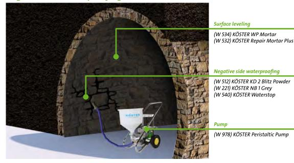
Several waterproofing systems can be applied to the negative pressure inner side. KÖSTER KD 2 Blitz Powder and KÖSTER Waterstop can be applied to stop small leaks. Joints can be repaired with KÖSTER Repair Mortar or KÖSTER Repair Mortar Plus and KÖSTER NB 1 Grey can even be applied on surfaces as negative side waterproofing.
