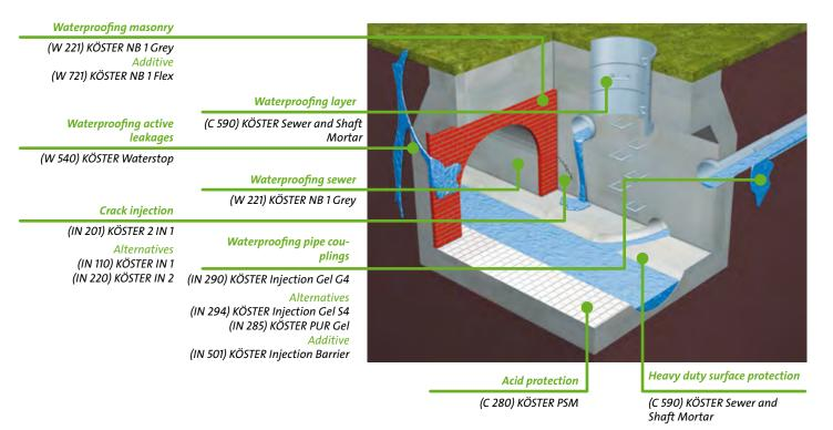
Water treatment facilities like sewage treatment plants, sewers and shafts or sewage water tanks made from concrete or masonry are exposed to a variety of stresses. The restoration of such facilities entails waterproofing, concrete repair and concrete protection as well as protection against acids and abrasion. For this a wide range of materials are used.
