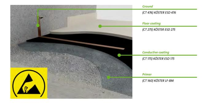
In areas where electronics are manufactured or in areas that can be electrostatically charged by people or machines, the floor must have a sufficiently high electrostatic dissipation to eliminate the risk of damage. For this ESD protection areas are required, (ESD : Electrostatic Discharge) where special ESD coatings are installed.
