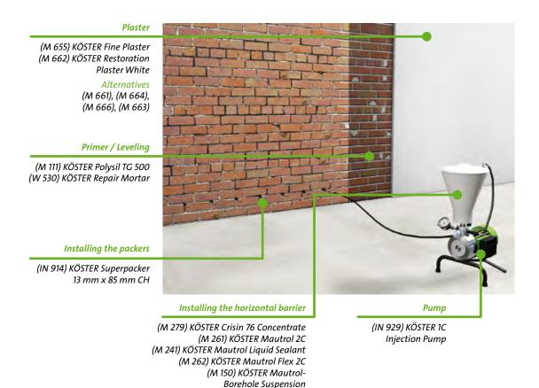
Fast and effective: The installation of a horizontal barrier via pressurized injection. When it is possible to ensure that the wall is free of cracks or voids, the horizontal barrier can be installed with a pressurized injection system. Cracks and voids which become apparent during the drilling process can be filled with KÖSTER Borehole Suspension. After filling, the borehole is re-drilled.
